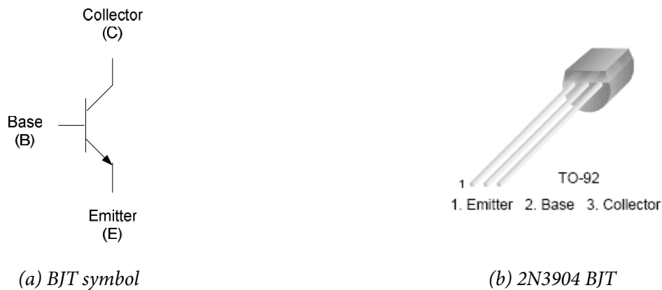
Figure 3. BJT symbol and physical appearance of 2N3904 BJT.
